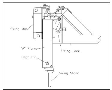
link tab to disengage the swing lock and loosen the chains to allow sharp turns again. This demonstrates how the top link of the tractor lift system switches the AERA-vator between the trail and lift modes.
