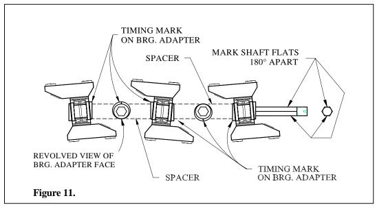
3. Install the required components in the sequence shown in Figure 11, double checking the timing mark locations and spacer lengths (see following table) as each rotor is installed.
