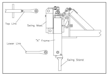
Figure 3. Hitch Adjustment
