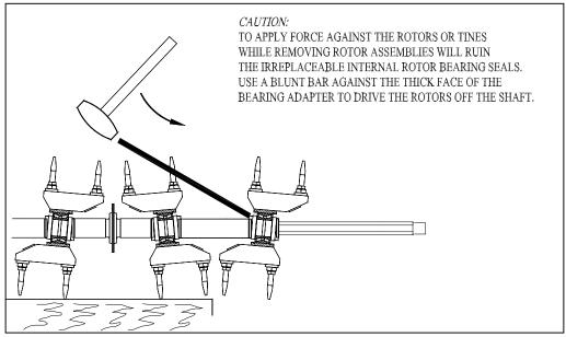
Figure 7. Rotor Shaft Disassembly
