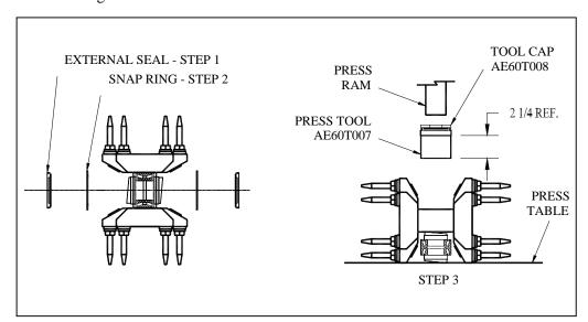
Figure 8. Rotor Hub Disassembly
