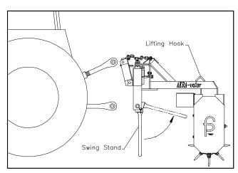
Figure 4. Swing Stand/Lifting Hook
