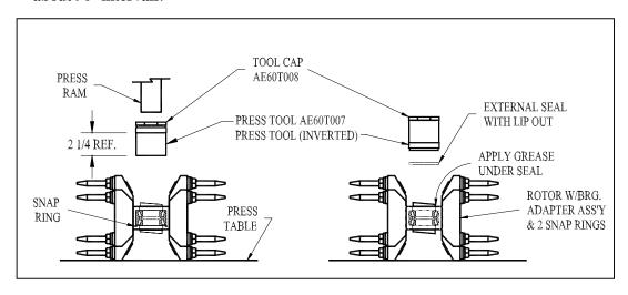
Figure 9. Rotor Hub Re-Assembly
