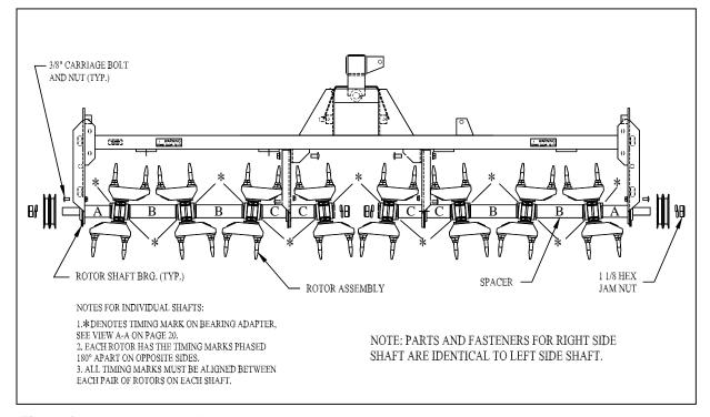
Figure 6. Rotor Shaft Assembly
